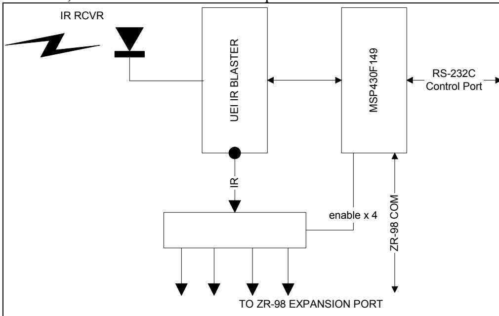
The MSP430F149 contains 60 kB of Flash memory and is used for storing a lookup table for IR Codes that are indexed by tokens sent from the ZAC-60. This offloads the storage requirements from the ZR-98 MotherBrain to the ZIR-232’s micro. It also minimizes storage and code requirements for the ZAC-60.
